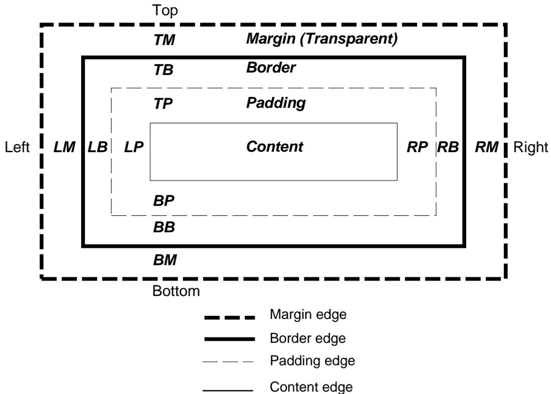
The margin, border, and padding can be broken down into top, right, bottom, and left segments (e.g., in the diagram, "LM" for left margin, "RP" for right padding, "TB" for top border, etc.).
