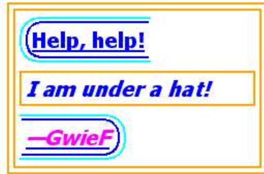
This diagram shows the boxes involved in the example above. The rounded aqua line represents the anonymous inline element wrapping the inline contents of the paragraph element, the rounded blue line represents the span element, and the orange lines represent the blocks.
