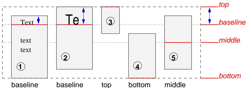
Diagram showing the effect of various values of 'vertical-align' on table cells.
