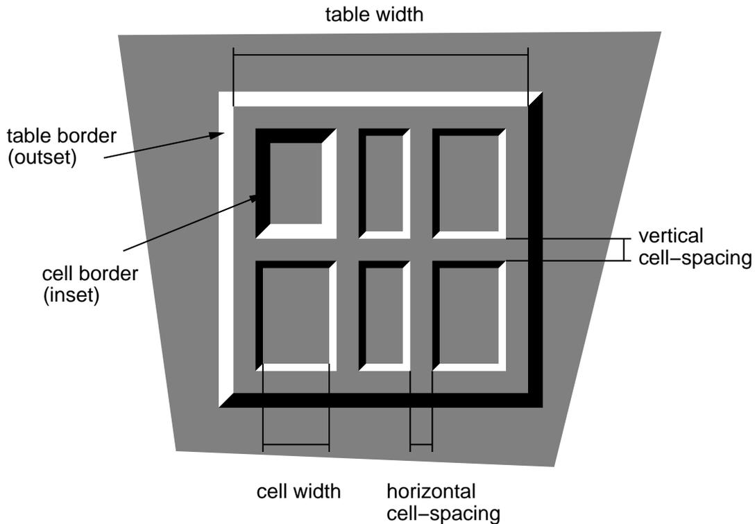
A table with 'border-spacing' set to a length value. Note that each cell has its own border, and the table has a separate border as well.
