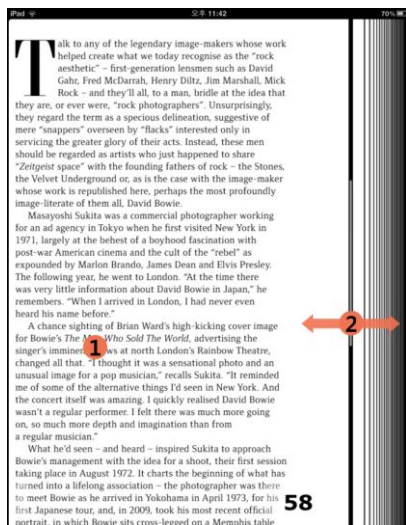
Figure 3. Initial touch“1” holds the page, second touch dragging“2” turns the page, releasing the initial touch either returns or stays in the remote page according to its released location or releasing direction
