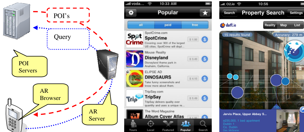
Figure 1: i) A typical system architecture for a "world browser" AR application. ii) A screenshot displaying available data layers from the popular AR browser Layar. iii) A screenshot from an AR application displaying local properties for sale from a popular Irish website daft.ie.
