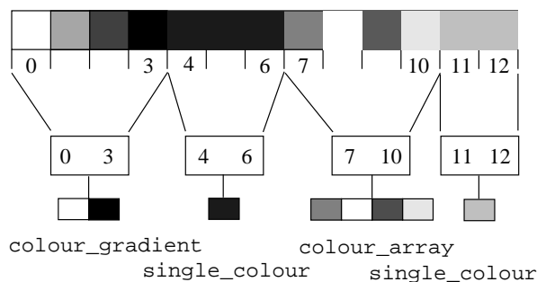
Figure 6: A pixel array (top) represented as a list of spans (bottom)
