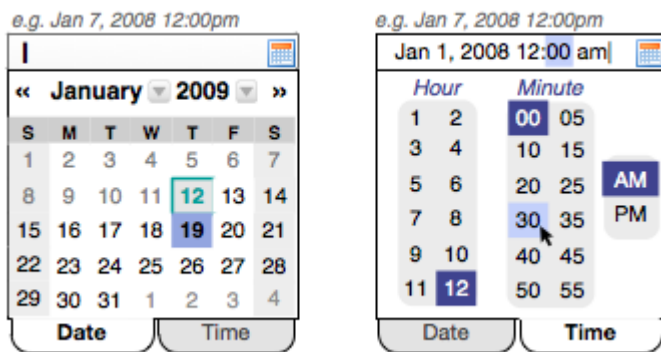
Figure 10: This illustration of an accessible date and time picker enables either selection of the desired date and time through entry in the text box or through manipulation of the mouse.
