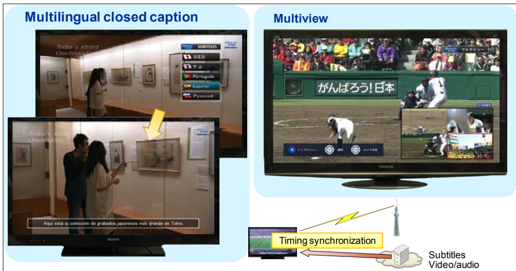
Fig. 2: Prototypes of services corresponding to use case 4. Additional content delivered via the Internet augments a broadcast program. (Left) Multilingual closed caption (Right) Multiview
