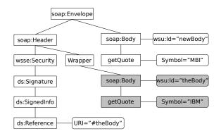
Figure 2: Example message after the attack. Parts of the tree processed by the signature verification algorithm are colored in gray. Parts of the tree processed by business logic are contained within "soap:Body".
